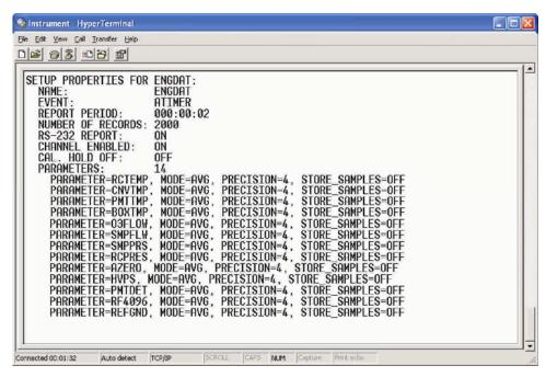
Figure 7-4: DAS Configuration Through a Terminal Emulation Program
